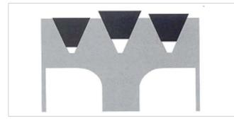
Frictional engagement between the lateral wedge surfaces require a large cross-section and high stiffness of V-belts
