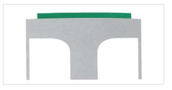
Frictional engagement on the outer pulley surface require only a small cross-section and make flat belts very flexible
